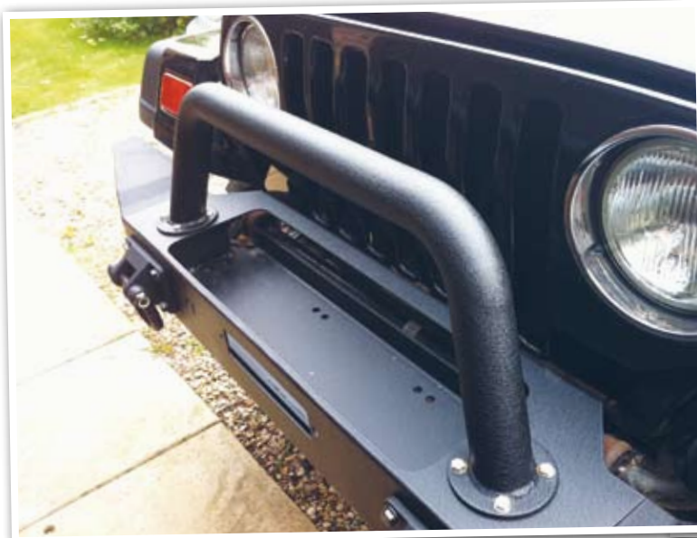
Substantial Rugged Ridge XHD bumper comes predrilled for industry standard winch sizes
