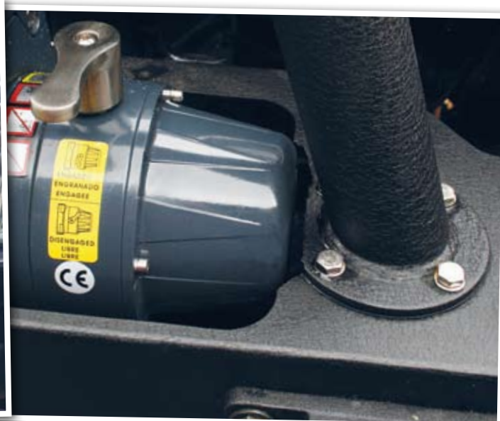
A small amount of trimming was needed to accommodate the brake housing
