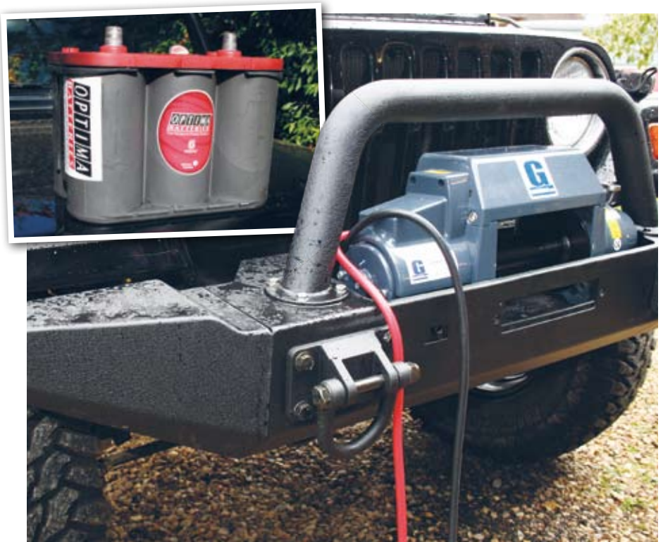
TDS installation is easy just run the power to the battery, solenoids are prewired. Inset: Superb Optima battery provides the muscle
